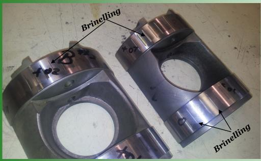
The two Sundstrand 90series—055 swash plates above have been successfully ground and the final size measured with special measuring equipment sourced from over seas.
